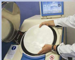
Ejection of disinfected disk evacuated directly into domestic container
